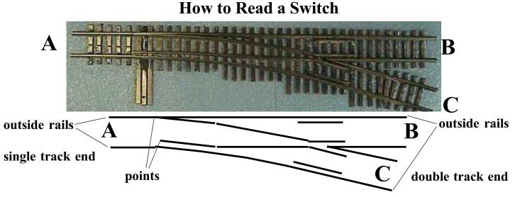
At the <u>single track end</u>, one point will be closed (touching an outside rail), and one point will be open (not touching the outside rail). Follow the outside rail <u>where the point is open</u> (not touching) to determine which way the train will go. In the case above, trains can move from "A to C" and "C to A". Trains coming from "B" will derail (hop off the tracks and crash).
